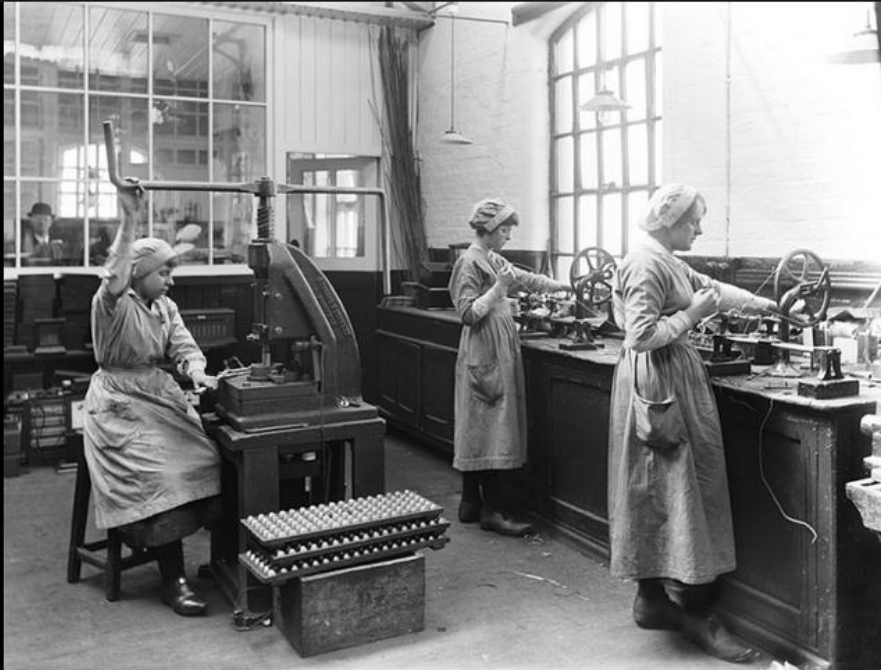
Women workers in the telegraph shop at Horwich works, May 1917. They appear to be manufacturing nose caps for artillery shells, using machinery made by Rhodes & Sons of Wakefield. A bowler-hatted foreman oversees their work through the windows of his office next door. Picture: © National Railway Museum/Science & Society Picture Library
